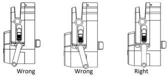
Clamp the tube straight into the grove as per above image in order to avoid the tube to cut through during the run.
