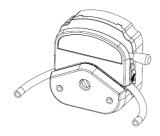
Make sure the lever is completely locked in order to ensure that there is enough pressure to hold the tube into position and to avoid the tube to become loose during the run. It is recommended to check the flow rate with water before adding the experimental fluids.
